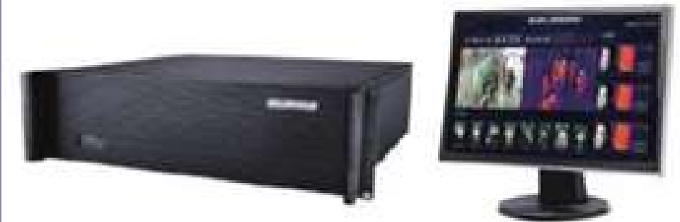
Temperature analysis processing module
