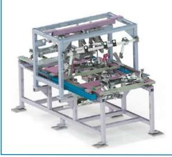
A global tier 1 automotive component manufacturer needed to verify dimensional quality of engine cradles in an inline process. The application required 32 feature inspections in under 13 seconds to meet high-volume cycle times and adherence to strict GD&T (Geometric Dimensioning and Tolerancing).
