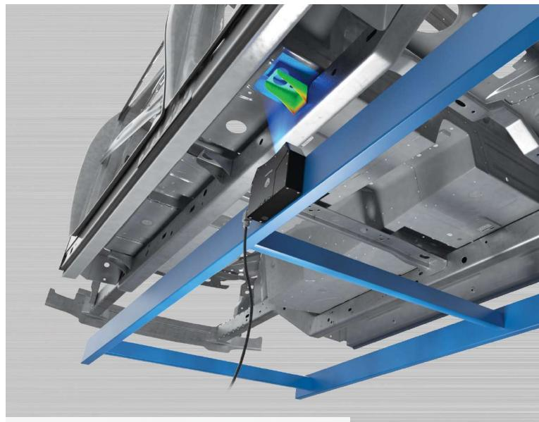
In underbody inspection, a snapshot sensor is used to scan features that a robot cannot reach
