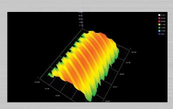
A structured light scanner digitizes an entire area into a 3D point cloud by projecting several light patterns in a rapid sequence onto a stationary surface. These systems can be mounted onto robots for flexible inspection applications, or to inspect larger objects like automotive panels by taking multiple snapshots from several zones.
