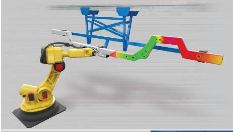
Ensuring sideframe mounting holes are the right size and in the right position
