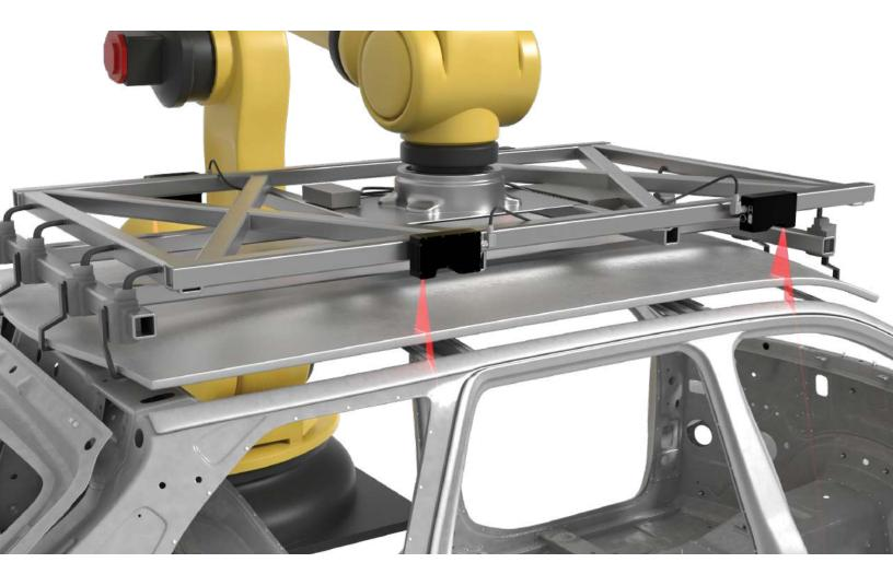
Automation presents a number of challenges for quality control in the automotive industry. These factory processes require an advanced 3D machine vision solution to maximize efficiency, lower cost, and increase yield.
