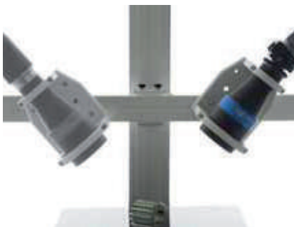
Scheimpflug telecentric optics for both projecting and imaging at 90°.
