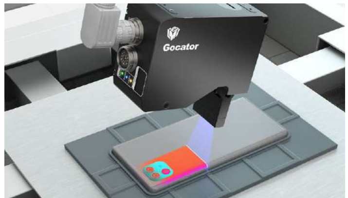
Gocator® 2522 scanning cell phone cover glass assembly
