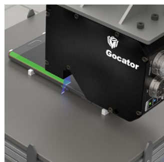
Phone bezel gap and flushness
